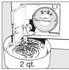
■ Turn the lint trap lid counterclockwise 2 - 3 times. Do **not** remove it. About 2 quarts of water will drain out of the hose.
